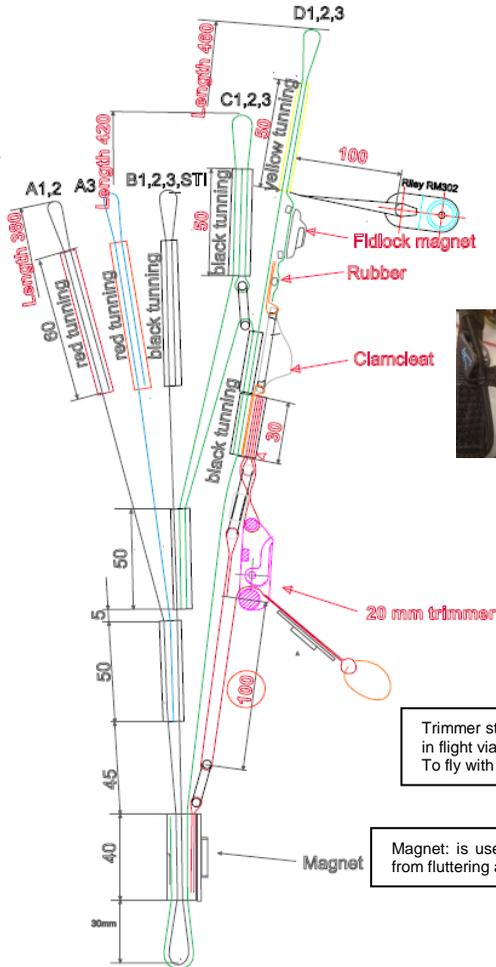
**Fidlock:** to fix the brake handles when folding the glider
