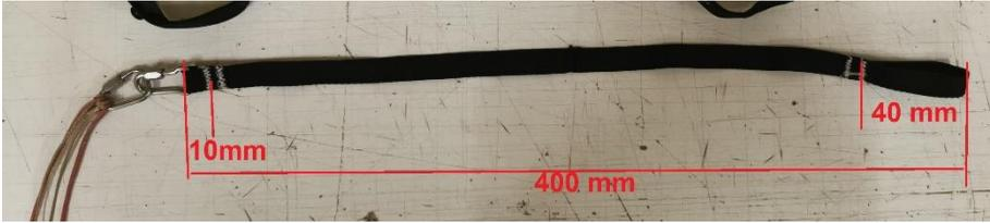
Attach the quicklink to a 15mm polyester strap (15mm / 0.5mm) with loops as shown in the illustration with another quicklink.
