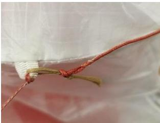
The folding lines fa13 and fa14 are attached to the respective line attachment point with the folding line loop (loop length is 20mm).
