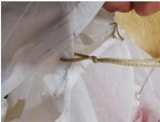
For the additional folding line loops, carefully pierce the leading edge of the sail behind the crossing of the rods. Then thread the "f-loop" line with a splicing needle and knot the "f-loop" line with a loop length of 20mm. This affects the folding lines fa1 to fa12. After removing the folding line loops, the resulting hole must be taped on both sides with a piece of adhesive sticky cloth.
